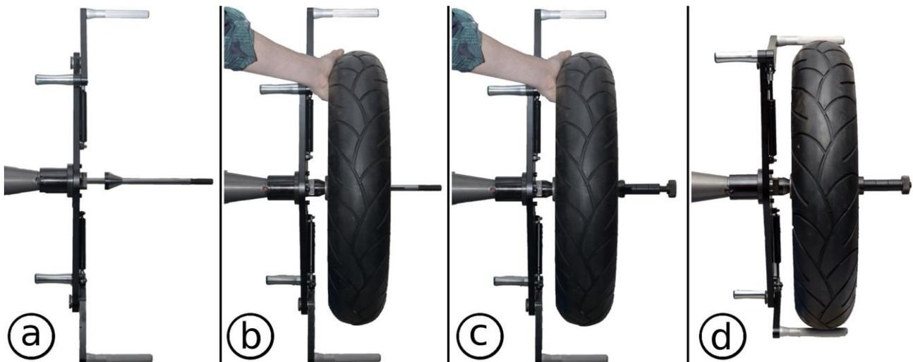
*fig. 5.13 Mounting motorcycle wheel on the holder.*
