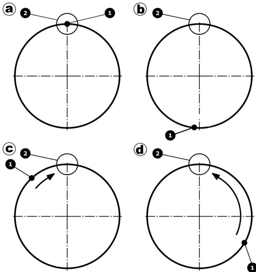
fig. 6.8 – Weight placement correction: 1: firstly placed weight
