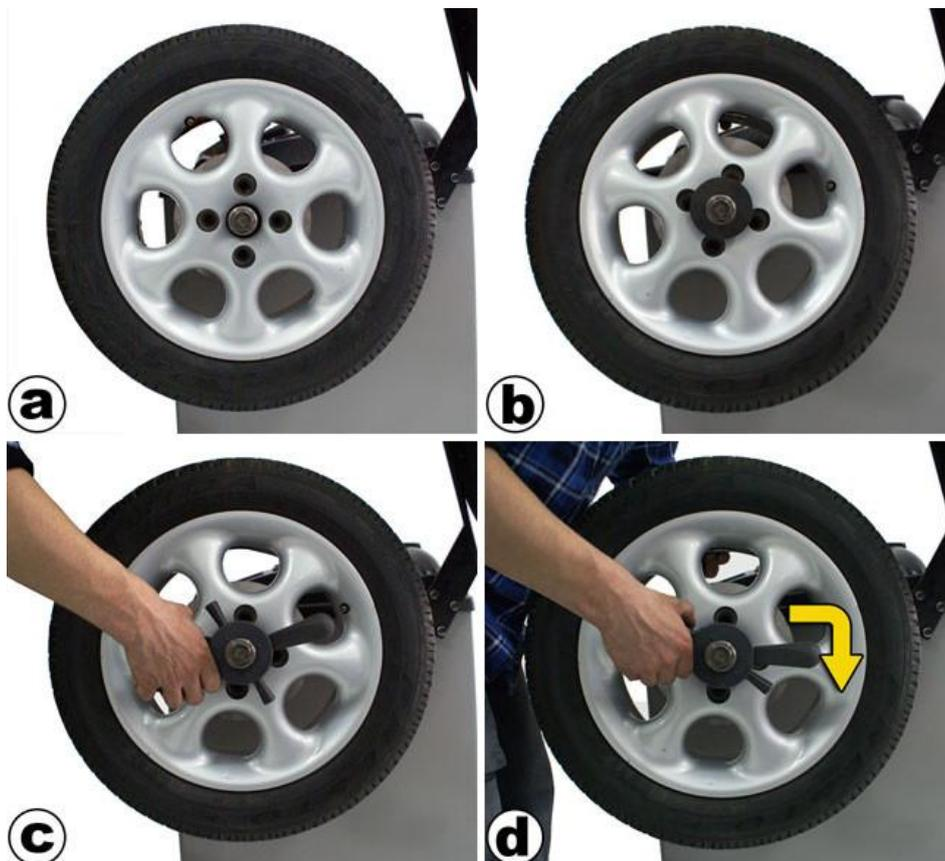
Fig. 5.7 Mounting a car wheel in the holder.
