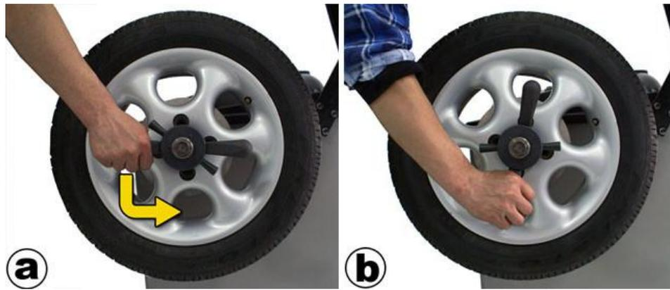
*Fig. 5.8 Dismounting the wheel from the holder.*
