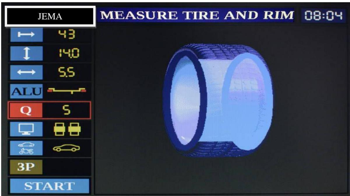
Fig. 6.12 – Optimisation screen – tyre and rim measurement
