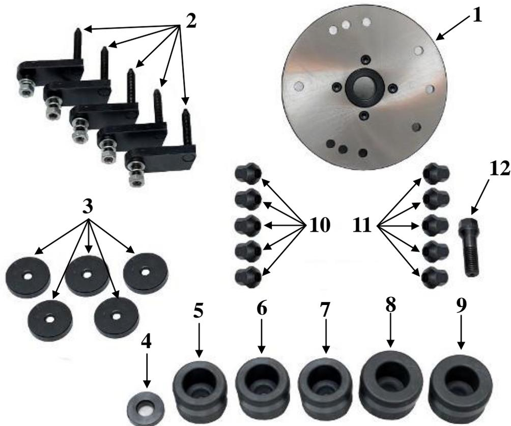
*Fig. 5.5 Spike holder's elements: 1: holder's disc 2: spikes for wheel mounting 3: plates 4: pad for mounting bolt 5: centring muff  $\phi 55$  6: centring muff  $\phi 56$  7: centring muff  $\phi 58$  8: centring muff  $\phi 60$  9: centring muff  $\phi 65$  10: cone screw 11: spherical screw 12: bolt used for mounting the holder on the spindle*
