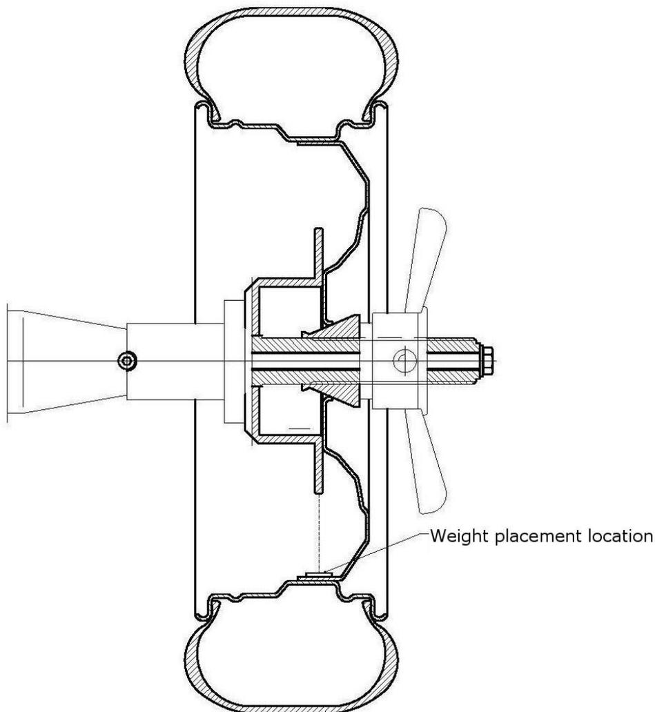
*Fig. 7.4 Weight placement location for adjuster's EASY mode.*
