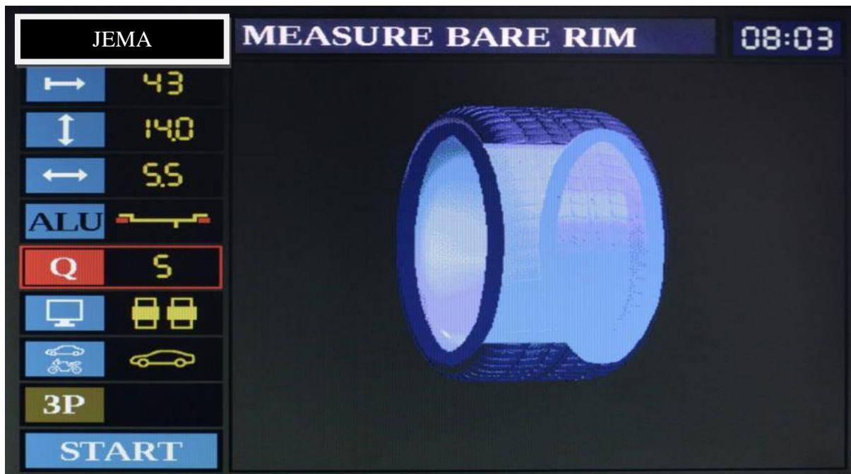
*Fig. 6.10 – Optimisation screen – bare rim measurement.*
