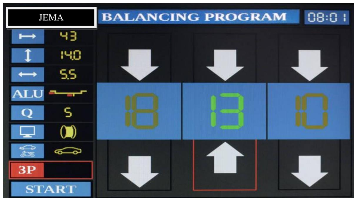
Fig. 6.7 – “Hidden weight” function – final screen.
